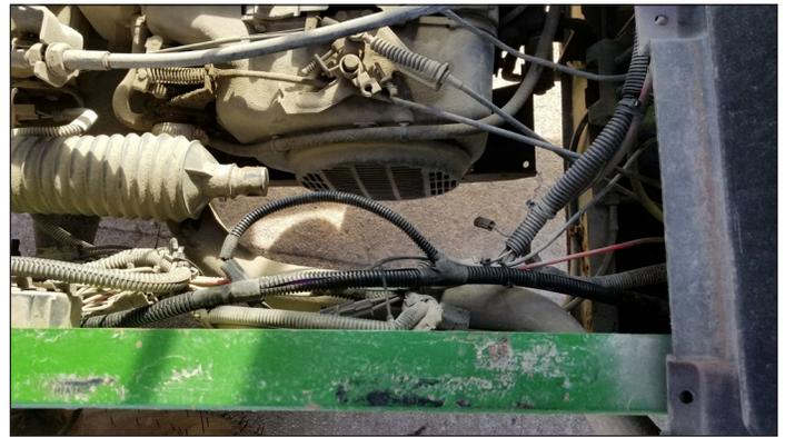
7. Connect the 2 pin connector (E) on the power harness to the rear attachment port connector (F) on the inside of the right frame rail.
