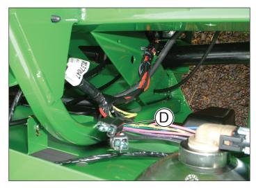
Raise the cargo bed and route the other end of the power harness from the battery compartment into the engine compartment on the inside of the right-side frame rail and lightly secure to the vehicle harness with a wire tie.
