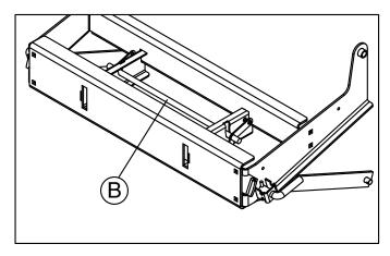
To release an attachment, lift rod (B) and slide the attachment forward slightly. This will unlock it, enabling it to be pulled out.
