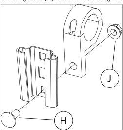
11. Attach the p-clamp to the left side of grab bar in the glove box. Do not fully tighten.
