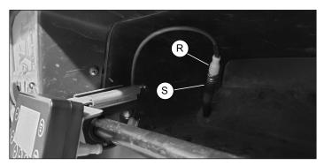
15. Adjust angle of display as best suited for operation and tighten p-clamp to grab bar.
