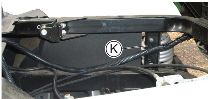
10. With the bed raised, run the 12 foot extension along the bottom frame tube. Wire tie about 6 inches from the end to the vertical support (K) as shown.
