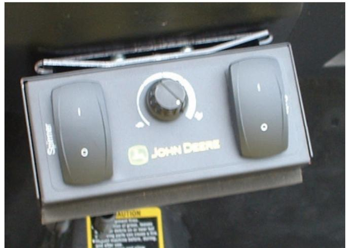
5. Slide the control box into the mount as shown. Connect the battery harness and 12 ft extension to the wires on the control box.
